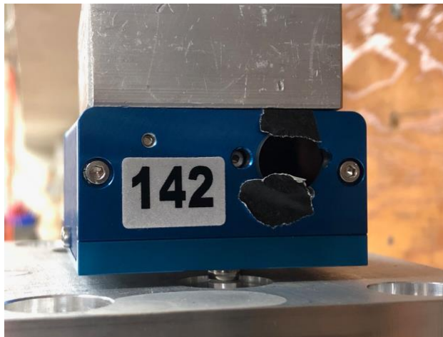
Figure 2 - Taping the neutral density filter over the NBCAM lens
