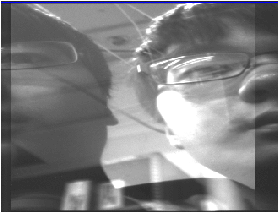
Figure 19: Distortion seen in an image taken by the ICX424Q with R_a = 200 \Omega .
