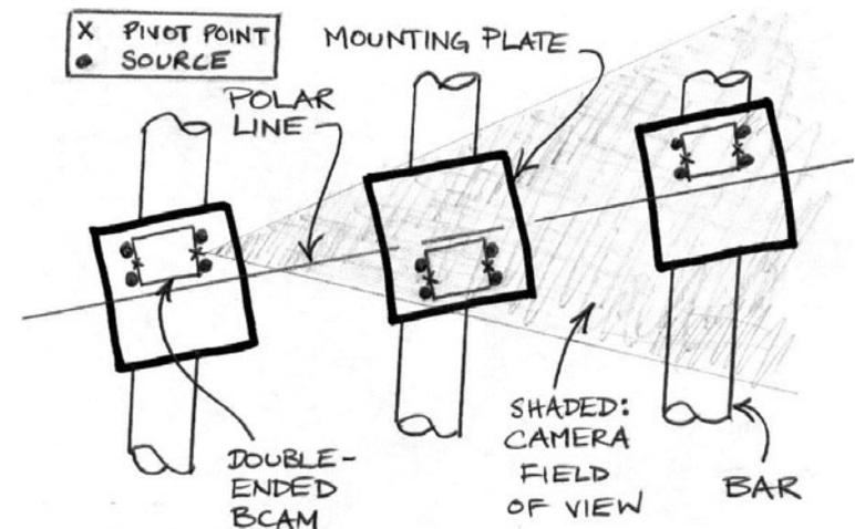
need both **absolute** and **relative** measurements because polar lines non-projective (not pointing to IP)
