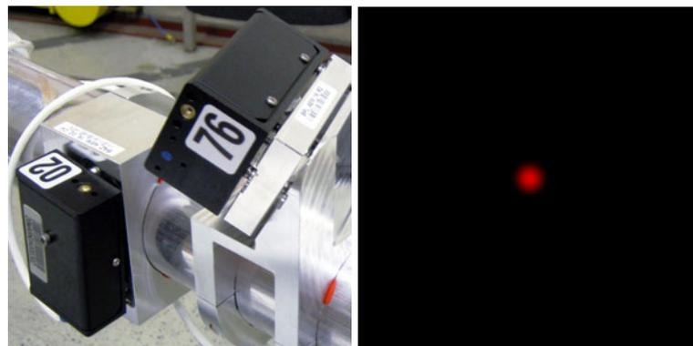
**RASNIK:** camera looks at coded chessboard mask, measures displacements
