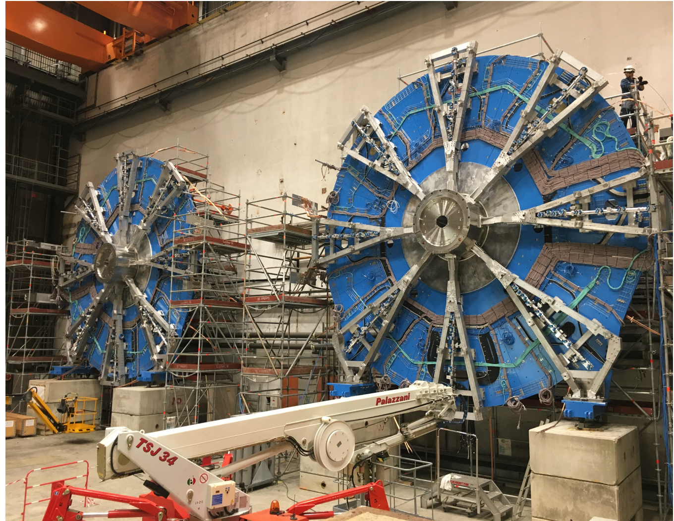
Small sector alignment bars mounted on A and C wheels
