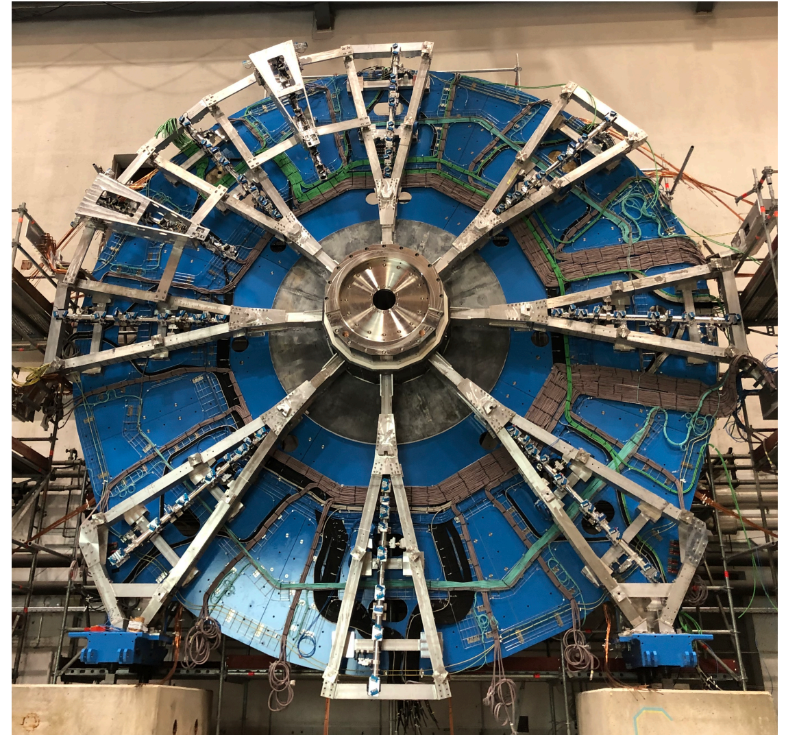
8 small and 2 large sector alignment bars mounted on C wheel
